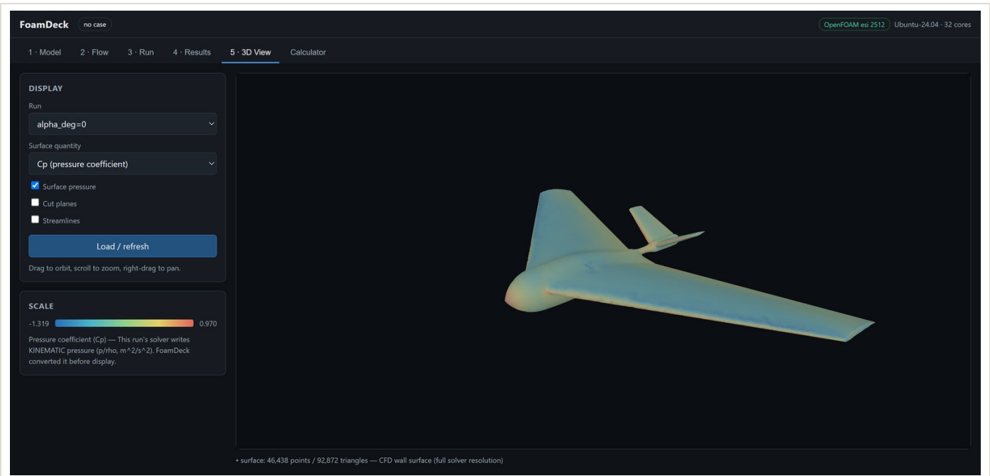
The GUI's 3D view: surface pressure coefficient on the analyzed aircraft.
