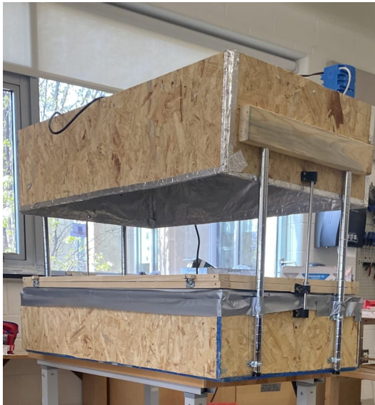
Full-size former: foil-lined heater box above the 2 × 4 ft forming bed.
